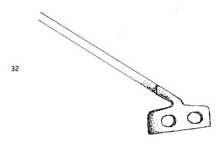
Mix concrete using a hoe. Any hoe will work, but the best hoes for mixing concrete are large and have double holes that provide twice the mixing action.
