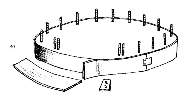
Remove the form boards once the concrete sets -- usually the next day. Provide a safe and clean job site by cleaning and stacking the form boards for future use.
