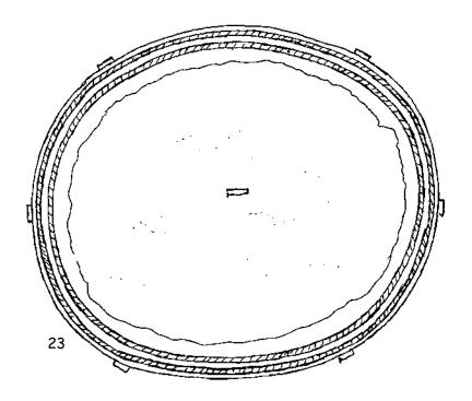
Place two continuous rebars 3/8" (10mm) in diameter into the trench. Rebars may be spliced with a 12" (30 cm) overlap.
