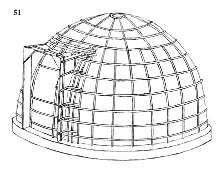
Place rebar around the augmentations and tie it to the shell rebar. Leave existing shell rebar in place; it can be cut out later. Use basalt rope or basalt rebar.
