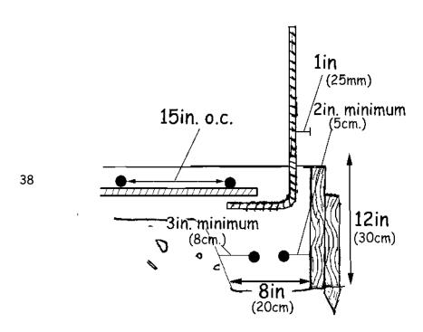
Placement shown is for an EcoShell with a 10' to 20' diameter. Larger structures may require different engineering. Always check for accuracy.
