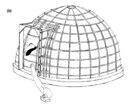
Position vertical rebars 10" (25 cm) apart. Place horizontal rebars over the outside of the vertical rebars. Attach horizontals to verticals. Please use basalt reinforcing. It will not be destroyed by rusting.
