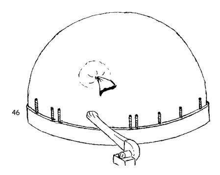
After all workers have exited, roll up and tie off the sleeve, making the Airform as air tight as possible. As placement of clamp angles progresses, ventilate under the Airform by starting the inflators. This is especially useful if a large fan is used only for this phase. The EcoShell Inflator must be used to properly inflate the EcoShell's Airform for construction.
