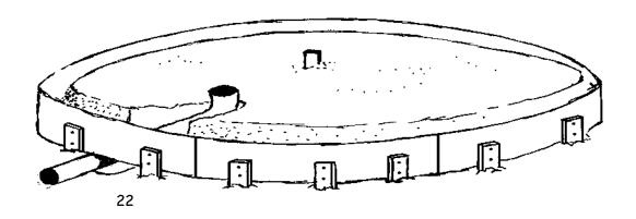
Slide pipe into the trench and up to its proper position.
