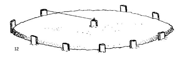
The floor will hold the Airform down as it is inflated. When inflated, the Airform for an EcoShell with a 20-foot (6m) diameter may have an uplift of 15,000 pounds (7,000 kgs).
