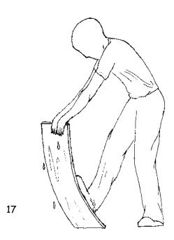
Manually bend the plywood. Before bending, the plywood may need to be soaked for a day or two. Usually, 1/2" (10 to 12 mm) plywood works best.
