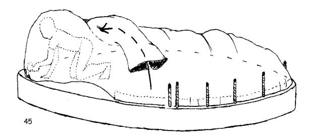
As placement continues, workers placing the clamp angles will wind up inside of the Airform. Workers can crawl out through the provided sleeve. A saw horse or other bracing device used to hold the fabric off the workers is helpful.
