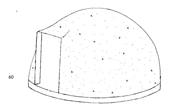
EcoShell is now structurally complete. Its exterior should be coated with an elastomeric coating to help with solar reflectance and to protect against possible leaks from hairline cracks.
