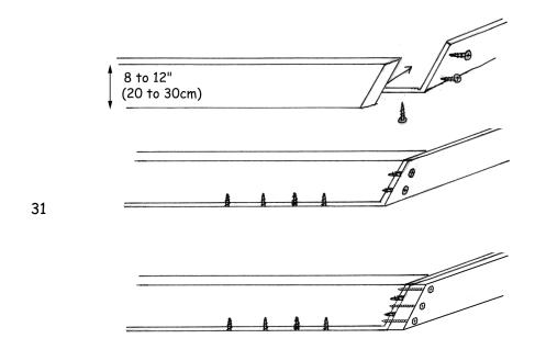
Fasten sheet metal to wood frames with screws or ring shank nails. To minimize leakage, place screws close together. First batch of concrete that's mixed will stop leakage.
