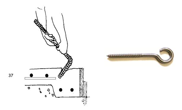
Important: Before the concrete floor/footing sets up, the uprights must be placed. Uprights are #3 rebar (3/8" or 10 mm). Place the short leg into the floor about 1" from the edge and turn it, as much as possible, toward the center.
