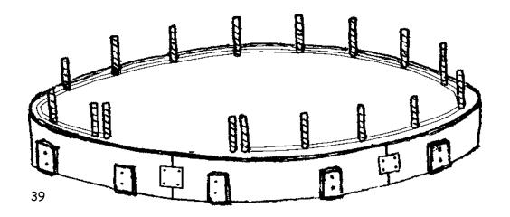
Place two uprights or hooks on each side of a doorway, but do not place any uprights within the doorway. Dig a small trench approximately 1" (25 mm) wide and 3/4" to 1" deep into the fresh concrete between the uprights, except for doorways. For larger structures, this trench should be 2" wide and 1" deep.
