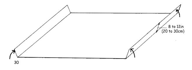
For 2 people, sheet metal measuring 36" x 72" (1m x 2m) is adequate. Factory bends can often be made at time of purchase. If not, the sheet metal can be field bent.
