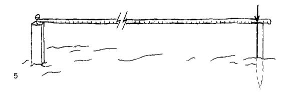
Set a nail into the middle of the center stake. Using a tape or pole, measure the distance from the center stake to points on the perimeter where the forming stakes will be placed.
