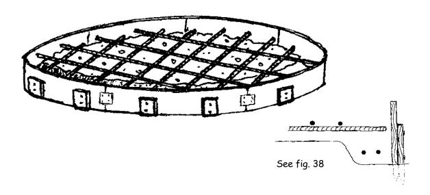
Place floor rebar in the middle of the slab. A cross pattern of #3 (3/8" or 10 mm or 6mm Basalt) rebar 15" (35 cm) on center is adequate for most floors. Stop rebar about 2" (5cm) from edge.
