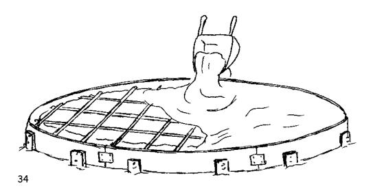
Use care in pouring the concrete so that rebar stays in the middle of the slab. Check to make sure that the placing of the concrete does not knock the forms out of alignment.
