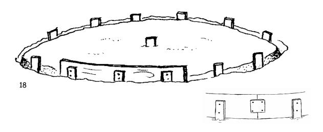
Place the formed boards inside the forming stakes and fasten them to the stakes, preferably with screws, but nails or staples can also be used. Fasten together the ends of the forming boards so that they will not move when concrete is poured inside.
