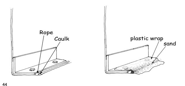
After all clamp angles are in place, the joints must be sealed. Clean the joints and seal them with caulking or with plastic wrap and sand. See last page for drawing of Clamp Angle.
