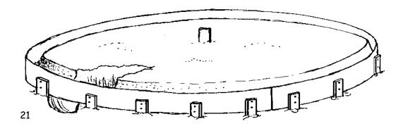
For plumbing, sewer or electrical installations, dig a trench under the plywood perimeter to the spot where the utility will be placed.
