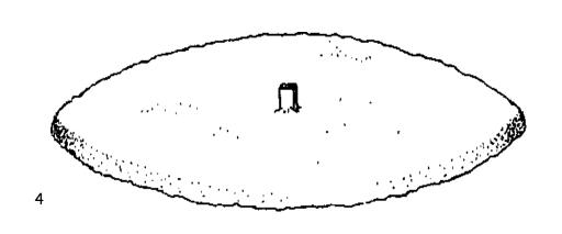
Set a stake into the center of the site that the EcoShell will occupy. This center stake will act as a guide for marking the perimeter.
