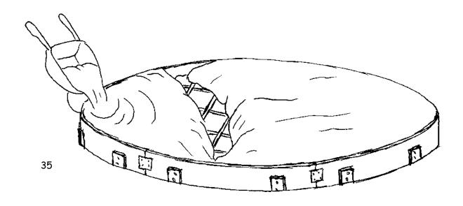
Place concrete. If placing of all of the concrete cannot be done in 15 minutes, start the concrete placing on one side and continue placing by moving across to opposite side.
