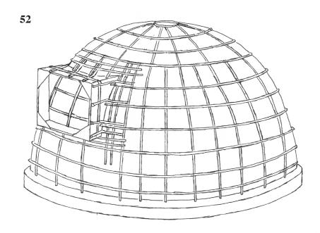
Place two or more extra rebars on top of and on the sides of the opening in the shell.
