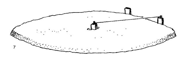
Space the forming stakes about 2 feet apart around the perimeter. That perimeter, created by the forming stakes, outlines the site for the foundation/floor slab edge of the EcoShell.
