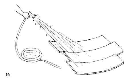
Wet the plywood. Wetting allows you to bend the plywood into the shape you need. If plywood is not available, multiple layers of a pliable material may be used.
