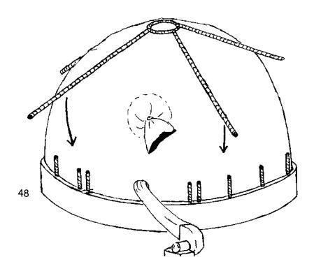
Tie the starter rebar to the uprights as shown, creating an even layout. Depending on the size of the dome, the layout will vary. Maintain a maximum spacing of 10" (25 cm) each way. Vertical rebar should lay against the Airform. Please use basalt rope or basalt rebar rather than steel.
