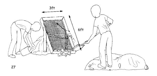
Sift the gravel by throwing the unsifted dirt at the top of the screen. As the gravel falls to the bottom, the proper mix size will fall through.
