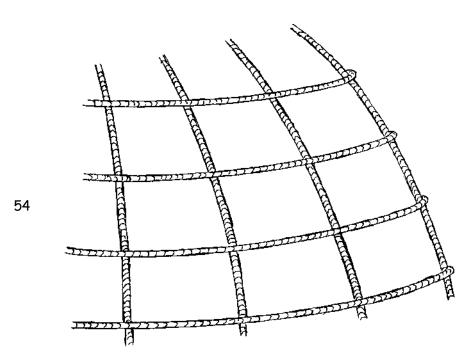
Make final inspection. Rebar should lay on the Airform with horizontal bars on the outside. Maximum spacing between rebar is 10" (25 cm) each way.
