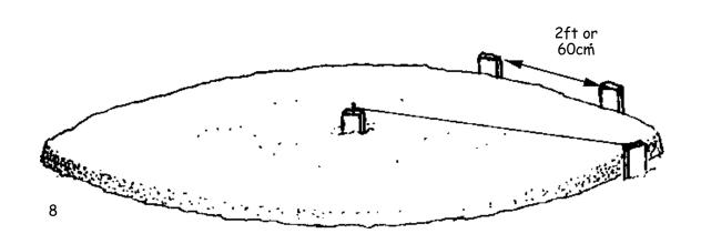
Drive the forming stakes deep enough so that they will hold under the concrete's pressure even after the footing trench is dug around the perimeter.
