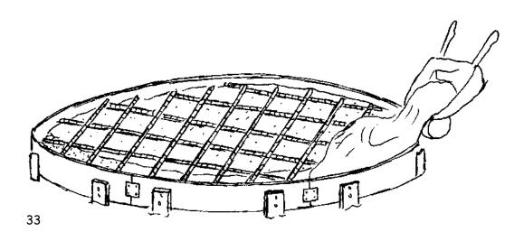
Mix concrete for the floor, by hand if you like. Concrete should be placed fast enough to prevent cold joints. Keep putting fresh concrete against older concrete all the way around.
