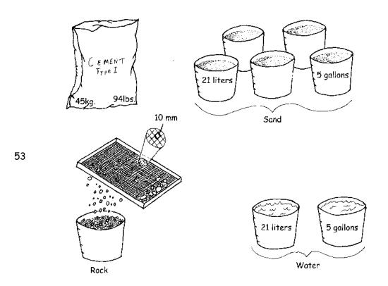
Shotcrete mix is stronger than the floor mix. It's designed as 4000 psi (280 kg/cm3) concrete. If sand contains coarse material, add another pail of sand and omit the rock. Add nylon fibers and Kel-Crete to the mix.
