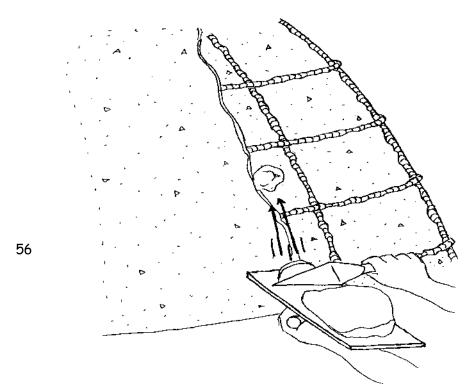
Note: A layer of concrete should be hard to the touch before applying a new layer of concrete over it. Be sure first layer is hard before applying second and second is hard before applying third. Keep concrete moist between coats.
