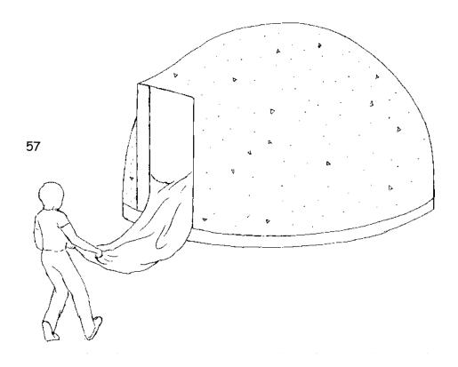
Remove the Airform after the exterior concrete has cured -- usually about 24 hours after the final concrete coat has been applied. But in cold weather, curing may take a few days.
