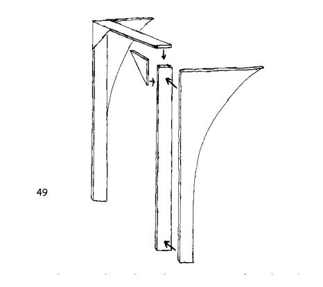
From plywood or boards, cut pieces that will make up the augmentations. Scribe them to fit the Airform. Then lean them against the Airform and fasten them to the rebar.
