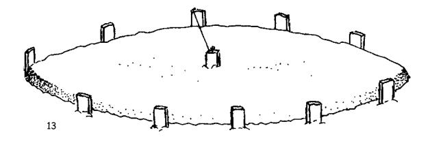
These instructions are for a small to moderate size EcoShell. Larger EcoShells may require deeper and wider footings. After the forming stakes are driven in and leveled, they should get a final diameter check.
