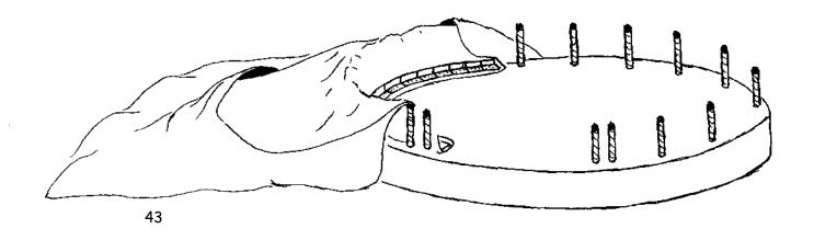
Continue placing clamp angles along the guideline. Carefully stretch the fabric along the guideline, distributing the fabric evenly all around. If not stretched evenly, there may not be enough to go all the way around.
