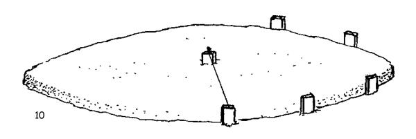
Check level and distance for each stake. Instead of trying to drive the forming stakes all to the same depth, mark the set stakes and cut them at the level you need.
