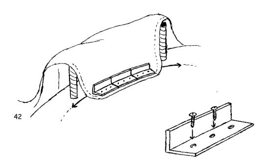
Place Airform as shown. Use 1, 2 or 3 concrete anchors as needed. Anchors can be screws (Tapcons) or a wedge foot anchor. It must be removable.
