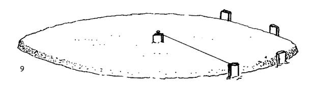
Remember that the forming stakes must all be at the same distance from the center stake plus the thickness of the forming boards. Center stake and forming stakes should all be at the same level.
