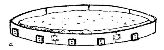
Check for proper trench diameter and be sure the floor is level. Keep in mind that changes/corrections are hard to make once reinforcing rebar is placed.
