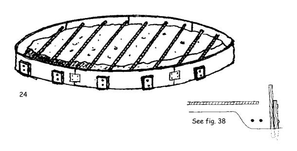
Use bricks to hold perimeter rebar (ring beam tendons) 3" off the dirt and at least 2" in from the formed edge. Then place the floor rebar.
